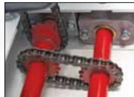
transfer box provides direct mechanical linkage between the barrier operator and spikes
